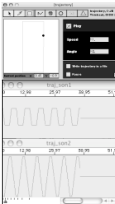
Figure 4. The coordinates of the rectangle trajectory on the top write themselves in the two buffers on the bottom. The upper buffer corresponds to the abscissa variation, the lower buffer to the ordinate variation.
